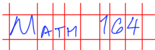
FIGURE 6. A rendering of the process of finding a bounding box for each drawn character. Each of these characters would then be recognized by a Kohonen neural network.
